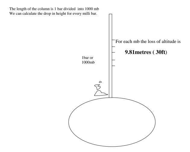
Using the standard we can calculate the pressure loss, due to altitude .
